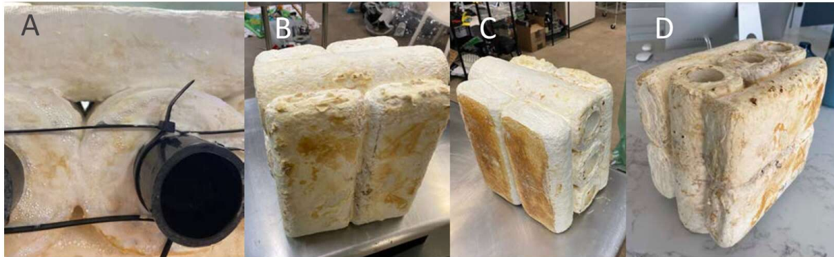
A) Detail of mycowelded parts. No adhesives required for bonding separate parts. B-D) different views of the finished, desiccated structure made from 7 different mycowelded parts of ZF
