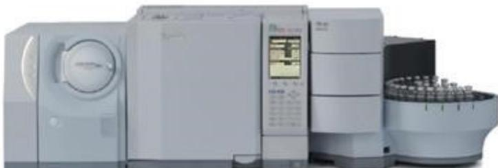
GCCM will use the Shimadzu GCMS-QP2010 Ultra with HS-20 Head Space Sampler and NIST spectral library to conduct comprehensive terpene analyses. The machine is capable of easily identifying over 3,000 flavor and fragrance compounds, which will meet all the company's terpene profiling and testing needs.
