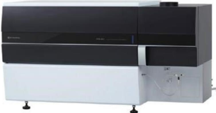
The company will use the ICPE-9810 Simultaneous ICP Atomic Emission Spectrometer to test for trace heavy metals such as lead, cadmium, arsenic and mercury to ensure all GCCM products are free from toxic concentrations of hazardous metals.
