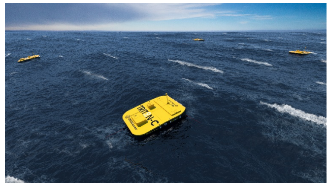
Sub-Scale Triton submerging under extreme wave conditions to reduce structural loads
