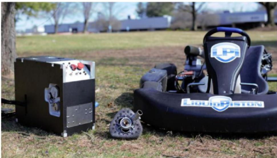
*Left: prototype 2kWe hybrid JP8 military generator prototype, powered by the X-Mini rotary engine*
