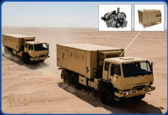
Artist rendering of 10kW Auxiliary Power Unit for next generation mobile command and control
